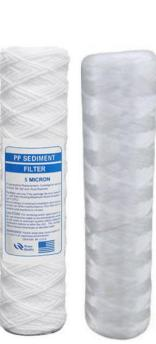
String Wound Filter Cartridge is a type of deep filtration filter element. It is made of textile fiber yarn (polypropylene yarn, defatted cotton yarn, etc.). These yarns are precisely wrapped around a porous skeleton (PP or stainless steel) to form a honeycomb structure that is loose on the outside and dense on the inside. These filter cartridges are widely used for liquid filtration to remove suspended solids, sediments, and other impurities.
