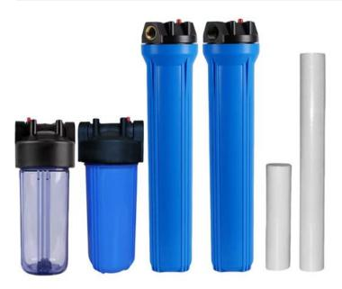
10" and 20" standard filter housings are constructed of a durable reinforced polypropylene or clear Styrene-Acrylonitrile (SAN). Filter housings will accommodate a wide range of 2-1/2" or 2-5/8" diameter cartridges. The reinforced polypropylene cap offers an optional pressure-relief button on the inlet side to relieve pressure inside the housing when changing filter cartridges. Polypropylene (HFPP) cap is available with 1/2" 3/4", 1" NPT inlet and outlet ports.
